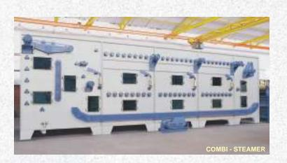
The **SWASTIK** Roller Bed Combi-Steamer (with Horizontal and vertical tight Strands) is designed keeping in view present day needs - a multi-purpose reaction chamber for a continuous Fabric Treatment Range for all kinds of fabric.
